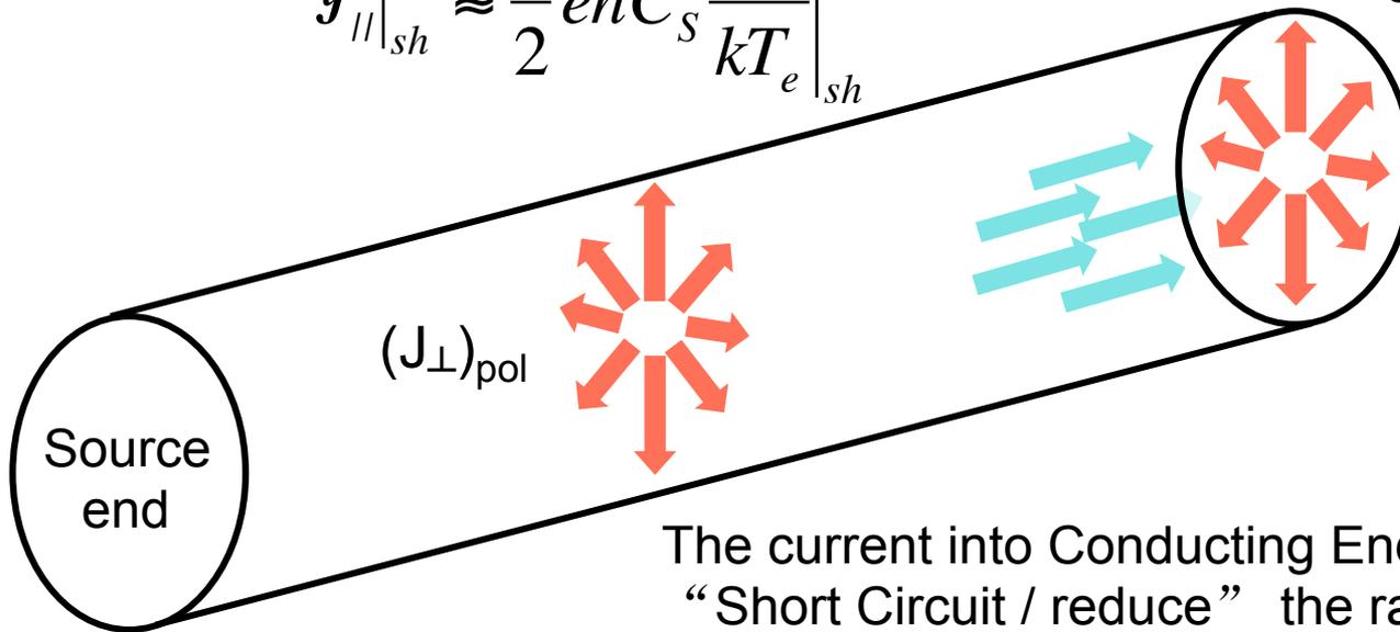
The current into Conducting End Plates can effectively “Short Circuit / reduce” the radial polarization current.
